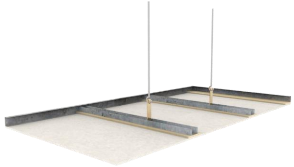
Non - Insulated Ceiling
