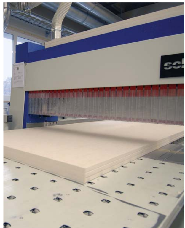
Cutting Promat boards with "Schelling 1" cut-to-size machine
