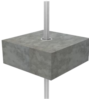
Up to 6x 3-core cables through a 50mm PVC pipe former in a 2 hour floor slab
