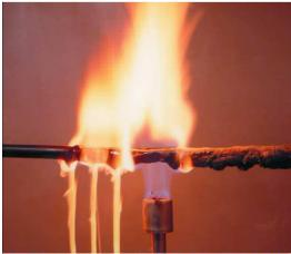
**PYRO-SAFE Flammotect-A** is an ablative cable coating product manufactured in Germany by SVT to protect cables from fire spread across their surface should a fire start on or adjacent to the cables.
